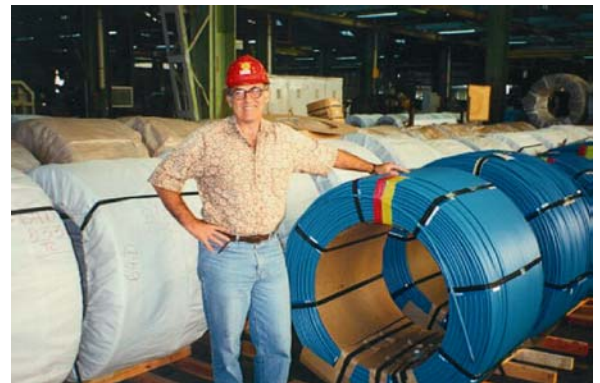
Fig. 2.5 – Cordoalhas engraxadas (Ref. Cauduro, E)
